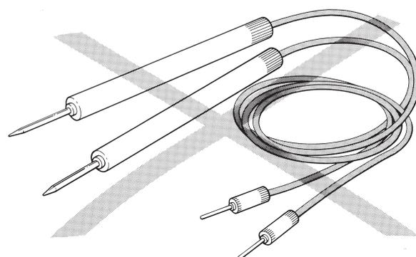
Figure 2 Test probes and leads (not recommended)
