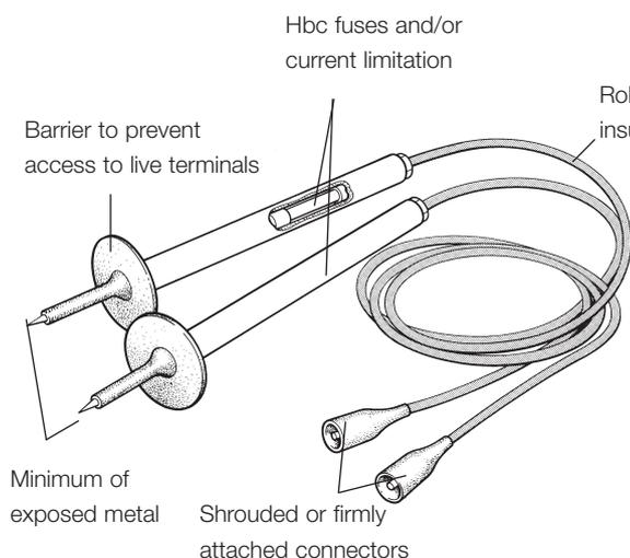
Figure 1 Test probes and leads (recommended type)
